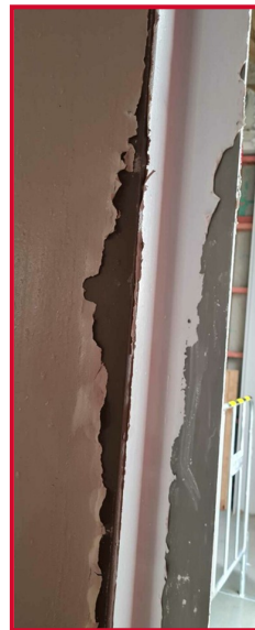
UNPROTECTED Solvent borne single pack intumescent with a fast drying, single pack, modified acrylic sealer
